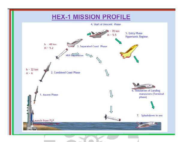
ISRO's RLV Technology Demonstration Programme (RLV-TD) is a plane-like reusable vehicle launched by an expendable single state solid booster. The mission will end with a splashdown in the Indian Ocean.
